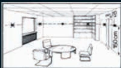
The thermostat should be located in the room where the heating is to be controlled, except in case of floor heating only.
