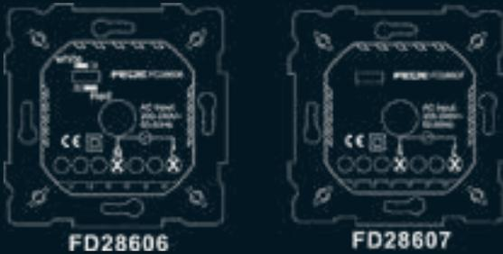
Connect the unit to the mains supply using the terminals on the back of unit.
